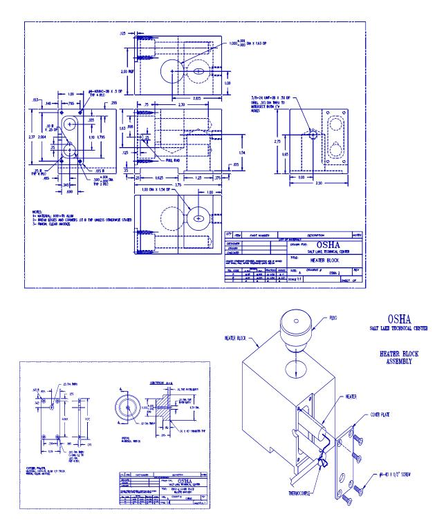
Figure 4: Engineering drawings for the aluminum "Hot Block" as used at the Salt Lake Technical Center.
